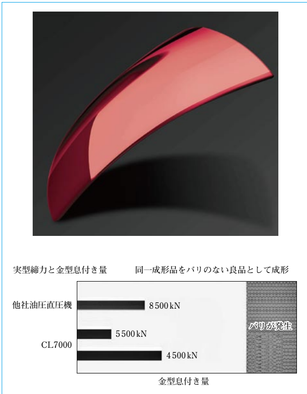
図6 アウターパネル成形品および従来機とCL7000の金型息付き量の比較 Molding part of outer panel and comparison of amount of mold movements for injection pressures of general machine and CL7000
