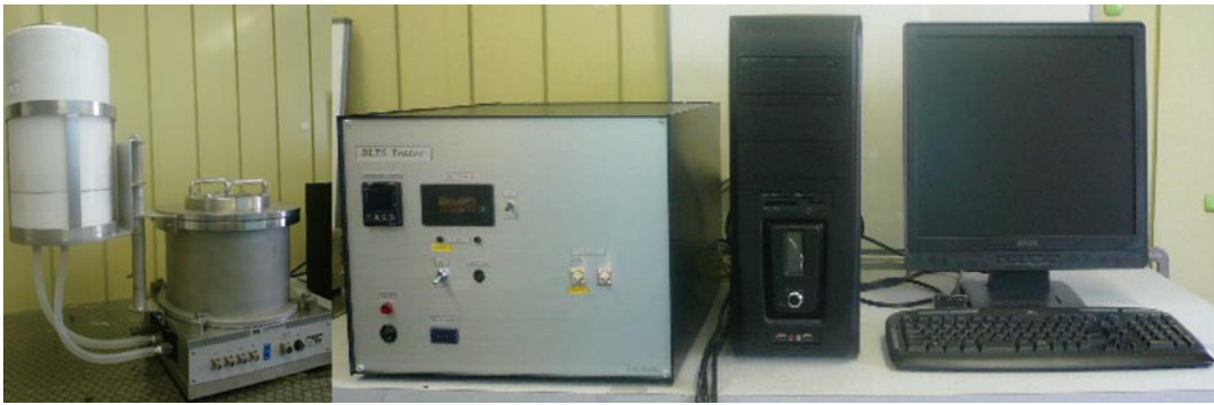
図2 DLTS装置 System of deep level transient spectroscopy
