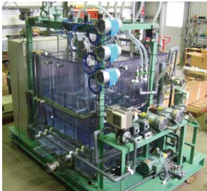
膜分離活性汚泥実証試験装置 Field test apparatus of MBR (membrane bioreactor)
