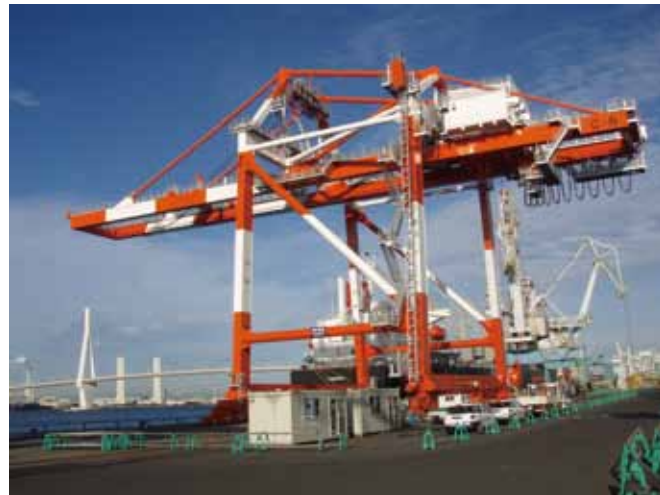
図7 製品荷役用橋形クレーン(BTC) Bridge type crane for product shipping
